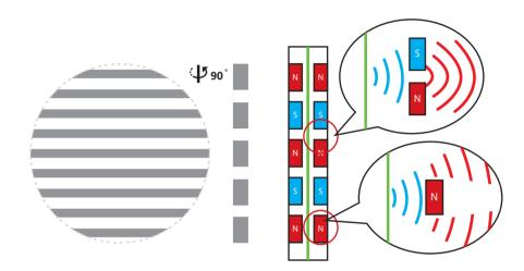
Unlike the sound waves created by a conventional magnet, the special shape of stealth magnet of HE1000se enables the waves to pass through the magnet without generating interference.
