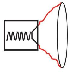
Conventional electrostatic headphone sees degradation of sound quality caused by the stator's interference.
