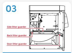
Remove white tapes inside and check if all the litter guarders are correctly attached. All the litter gaurders must be assembled correctly to prevent urine leaking.
