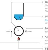
Short press to power on, long press to power off. Self-check of power on: 4 LED lights flash for 1 second then turn off. Short press the main device key to switch between SMART.
