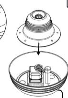
Insert the silicone cap and fold its top edge down over the top of the tube. This holds the cord in place and prevents leaks.
