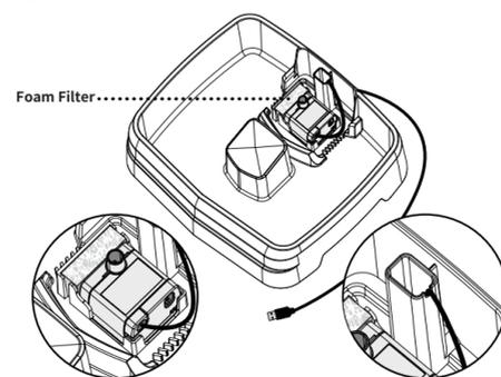
Put the pump and foam filter into the bottom of the bowl as shown. Press down to engage the suction cups.
