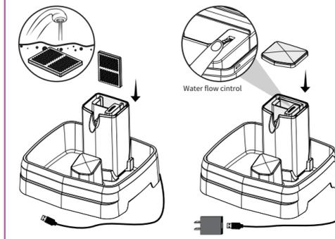
Insert the filter. The filter fits into the two slots located inside the tower.
