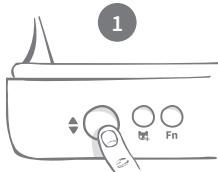
Press the open/close button (↔) to open the feeder.
