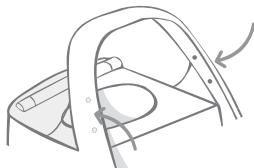
The feeder should be wiped with a damp cloth or household cleaning wipes. Make sure the four black dots on the hoop are kept clean to ensure reliable operation.
