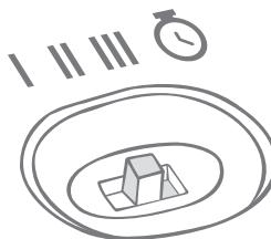
By default, the slider is set to the middle setting (II) for a standard delay time.
