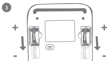
Insert the batteries. Ensure the +/- symbols on the batteries match the symbols on the feeder itself.
