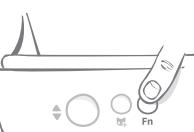
Start to increase the motion of the lid by pressing the Training Function (**Fn**) button once again. The lid will close a small amount and the light will flash orange twice.
