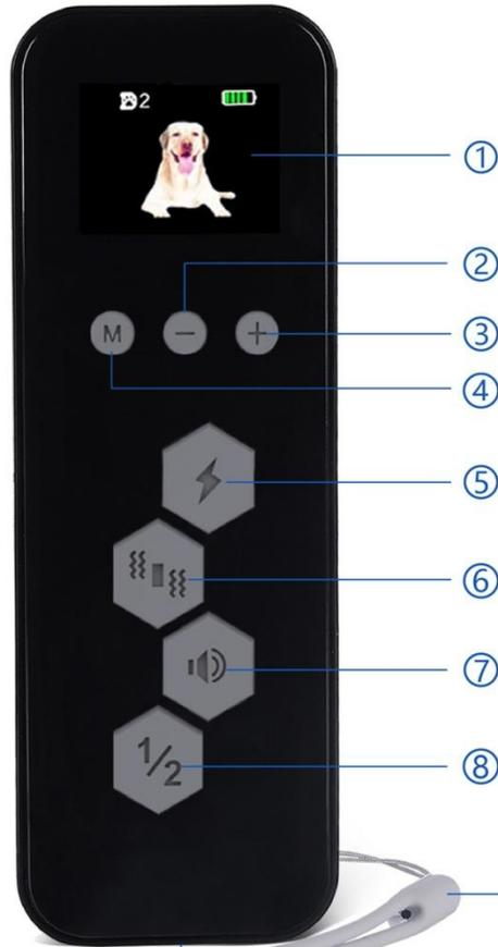
**1. Color Screen:** Color screen will display icons of dog, static shock, vibration, beep, Intensity, indication of battery and channel 1/2.
