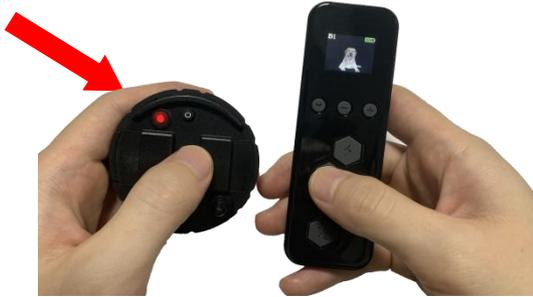
3. Press the "Static Shock" button on the transmitter, and you will hear "Beep" again which means this product has been matched complete. Use the test bulb to test the shock.
