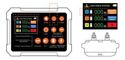
2. Gently press the switch button, and the screen will display the distance from the transmitter's central point to the fence boundary. Then, adjust the boundary distance by lightly pressing the "+" and "-" buttons. The boundary distance should be modified according to the size of your training area, ranging from a minimum of 10 feet to a maximum of 120 feet.
