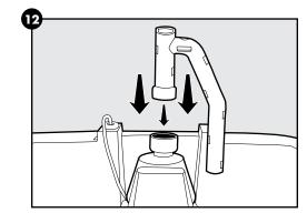
12. Insert the connector tube into the hole on the top of the filter housing as shown.
