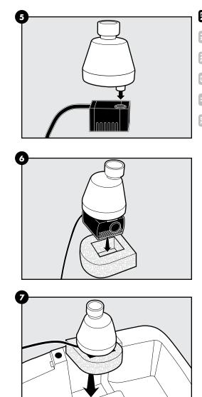
Place the assembled pump and filter housing into the foam filter with the cord running above it.
