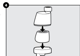
5. Insert the filter housing into the hole on top of the pump.
