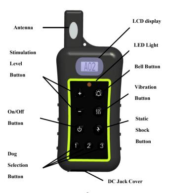
"and "buttons: Press these buttons to adjust the shock and vibration intensity from levels 1 to 10.
