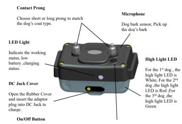
Press and hold on 4 seconds to turn the collar on. Two confirming tones will sound and the collar green LED light will flash 1 time per 5 seconds if connected. The LED will flash fast if disconnected. Press and hold on 4 seconds to turn the collar off. One long tone will sound and the green LED light will stop flashing and turn off.
