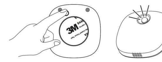
3. Peel off the 3M sticker on the back, place the air outlet downward, stick it to place where you expect and press it evenly for 10 seconds to get it secured.
