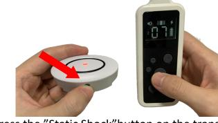
3. Press the "Static Shock"button on the transmitter, and you will hear "Beep" again which means this product has been matched complete. Use the test bulb to test the shock.
