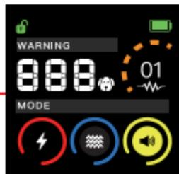
Lock: Press and hold the power button and the M button simultaneously. The screen will display the lock icon, and after 2 seconds, the device will be locked.
