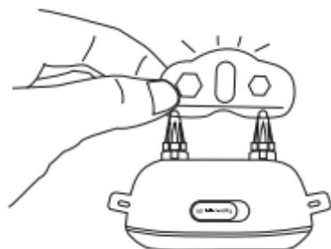
Turn on the bark collar and switch to Vibration + Static Stimulation Mode. Put the static test light on the contact points, then shout "woof, woof" to the collar while shaking it. Normally, the test lamp will flash when triggered.
