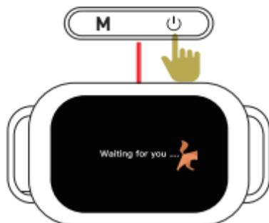
Press and hold the power button for 2 seconds to turn off. The screen will display "Waiting for you." The screen will then go dark.
