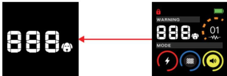
The product records a warning count every time it is triggered, starting at 001 and going up to a maximum of 999. To clear the warning count, press and hold the M button for 3 seconds.
