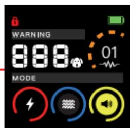
Unlock: Press and hold the power button and the M button simultaneously. The screen will display the unlock icon, and after 2 seconds, the device will be unlocked.
