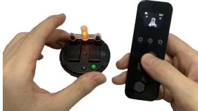
4. When the receiver does not work, it enters sleep mode after 2 minutes. Press any button on the remote control to reactivate it.
