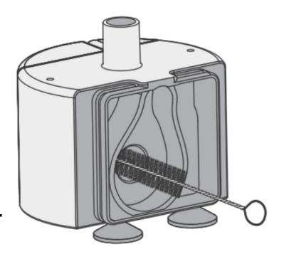
Clean the pump and fountain every two weeks. Remove the pump cover and rotor. Use a brush to clean the parts with water.
