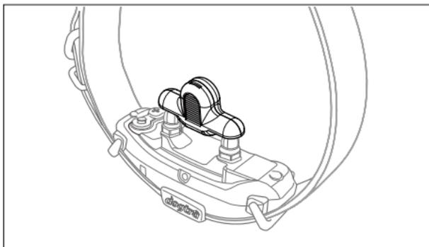
1. Turn on the receiver by touching the magnetic red dot on the back of the transmitter to the red dot on the receiver. The indicator light will come on for a moment then blink once every 4 seconds, showing that the receiver is ready to use.
