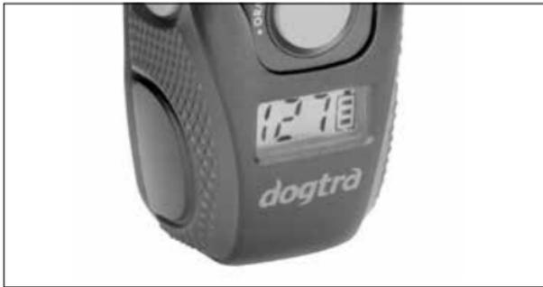
The LCD screen indicates the stimulation level on the screen ranging from (0-127). The battery life indicator shows:
