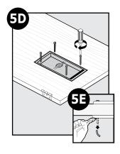
**5D** Use a screwdriver to evenly tighten screws throughout frame. It may be necessary to adjust screws to make sure pet door fit is correct.
