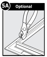
**5A Optional** Depending if your door is 1" thick or less, break away core frames of the interior and exterior frames. Use pliers to slowly and steadily bend down small sections across frame at grooved line. Go across the frame again in the same direction working the excess frame into a 90° angle. Next go back across frame in the opposite direction to slowly break off the excess.
