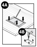
**4A** Hold the interior frame (the frame with the flap) in position. Mark the screw holes.
