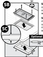
**5B** Place interior frame (frame with the flap) in cutout. Next place exterior frame into cutout from underside of the door. Hold frame pieces together with one hand.
