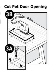
**3A** Drill %'' holes in inside corners of drawn template. These will be the pilot holes for the saw blade.
