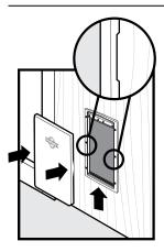
The Closing Panel snaps onto the interior frame of the Extreme Weather Pet Door™. It is useful during inclement weather or to keep your pet from using the pet door.
