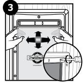
Replace flap clamp with attached insulated flap. Insert new vinyl flap between flap clamp and flap screw holes in top of frame. The PetSafe® logo should be readable on vinyl flap. Replace flap support. Align screw holes in flap support, frame, vinyl flap and flap clamp. Replace and start screws to hold flap in place. Adjust flap horizontally until centered in pet door frame. Adjust flap vertically until magnet bar on frame jumps to meet magnet on bottom of flap. Tighten screws.
