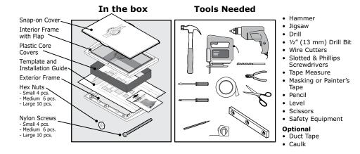
NOTE: The Extreme Weather Pet  $\mathsf{Door}^{\bowtie}$  can be installed in most doors and walls. Installation in thinner or thicker applications may not require the Plastic Core Covers. If installing in a wall, reduce cut-out width by 1" for the Small and Medium. For the Large reduce cut-out width by 1" and cut-out height by 1". Additional tools and materials, such as wood framing, may be required.
