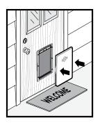
An additional closing panel (sold separately) can be used on the exterior frame of the Extreme Weather Pet  $\mathsf{Door}^{^{\bowtie}}$  for improved weather resistance. See "Replacement Parts and Accessories" on page 10.
