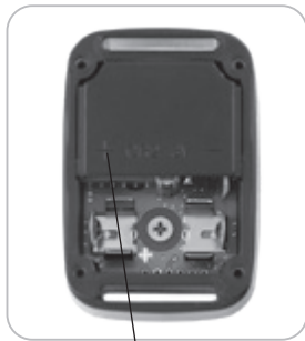
Battery polarity mark
