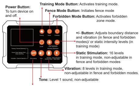
Pairing Button: Or the Switch button serves multiple functions:
