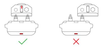
Training Mode: Attach the static test light and press the static button to test its functionality.
