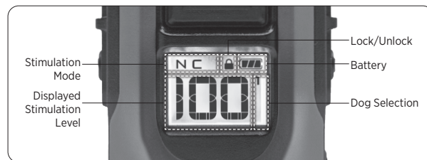
640X Transmitter LCD Screen
