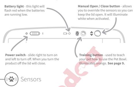
The sensors on your Sealed Pet Bowl will react to any physical movement within their range and are positioned in three separate locations to detect your pet approaching.
