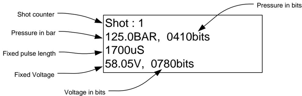
The shot counter will increment with every shot and the pressure will drop accordingly. Both the pulse length and voltage parameters are fixed and shown in decimal notation and in bits for convenience. If the gun does not support voltage programming (only later Mk5 GCUs and onwards support this feature), then the bottom line is to be ignored.
