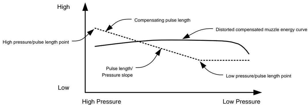
Ideally the compensating pulse length needs to be non-linear, unlike the straight line slope used in in SS compensation. This is done by introducing a dual slope that approximates the required non-linear pulse length/pressure curve, this is shown below:
