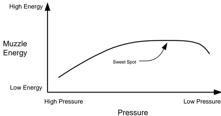
Because muzzle energy is largely proportional to valve hammer energy which is also largely proportional to pulse length, the power curve can be straightened out if the pulse length is increased in proportion to pressure as shown below:
