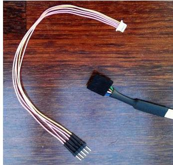
The five wire adaptor is used to connect the more recent guns, the single colour coded wire indicates Pin1 and must be plugged into the empty position on the larger connector to give the correct polarity. See below for a labelled description of the cable assemblies:
