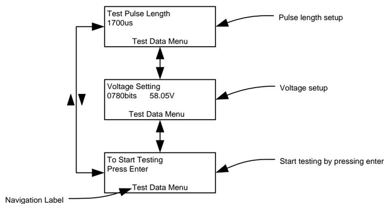
These Test Pulse Length and Voltage Setting screens allow pulse length and voltage to be reviewed and edited before starting the setup procedure. Pressing enter while in the bottom screen will program the edited values shown in the previous screens and put the gun into test mode. When the trigger is pulled the following screen will be displayed:
