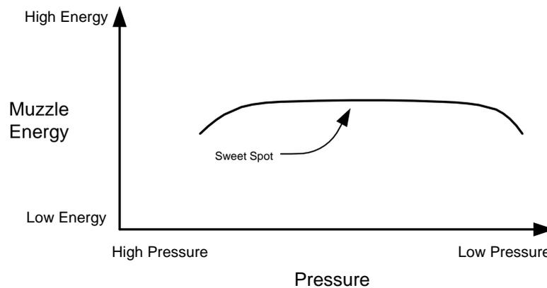
The principal goal of the setup procedure is to set the pulse length for the required power level at the middle of the power band at the "sweet spot" as shown above. This is most important for sub-12FPE guns where gun shall not be capable of producing more than 12FPE. The procedure to do this is listed below:
