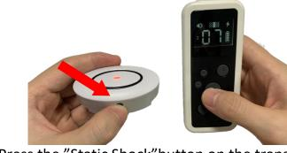
3. Press the "Static Shock"button on the transmitter, and you will hear "Beep" again which means this product has been matched complete. Use the test bulb to test the shock.
