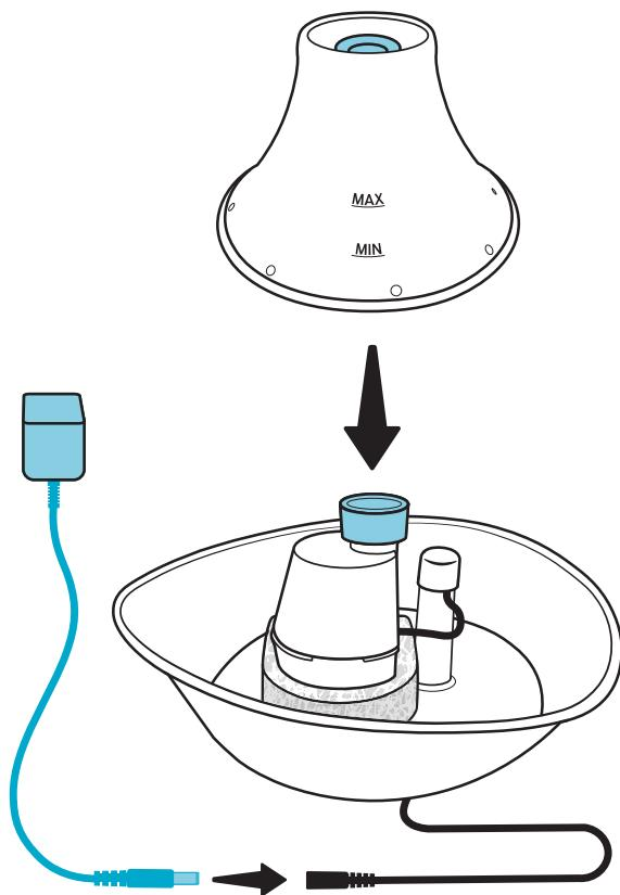
**EN** Set the tower down over the filter housing and press down on the silicone gasket to form a seal. Connect the power adaptor.
