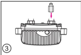
**Step 3:** Screw the metal prongs onto the receiver till the prongs are securely attached. Normally, they are assembled in the factory.
