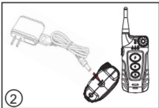
**Step 2:** Charge the transmitter. The signal light will flicker until battery is fully charged.
