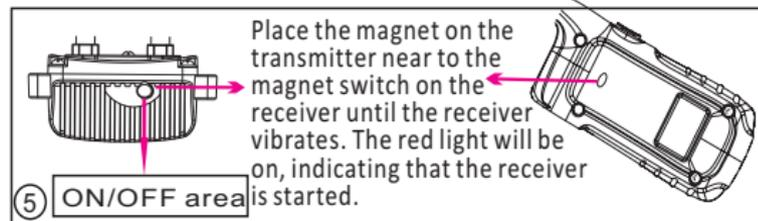
**Step 5:** Turn the receiver on/off. Bring the magnet on the transmitter near to the magnet switch on the receiver until the receiver vibrates. At that time, the red light will be on/off, indicating that the receiver is started/off. If you just finish charging, unplug the charger, and the receiver is on already.
