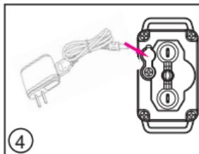
**Step 4:** Charge the receiver. The RED LED light of the receiver will be on while the receiver is charging. When the receiver is fully charged, the BLUE LED will be on. Once you unplug the charger, the RED LED light will stay solid on-waiting for sync. At the same time, the Blue LED light will go off.
