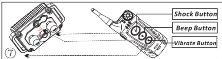
**Step 7:** Check the button functions. Push the beep button, and the receiver beeps. Similarly, press the vibrate button, and the receiver vibrates. Cap the shock test kit on the metal prongs, and press the shock button. If the bulb lights up, the shock function is normal.
