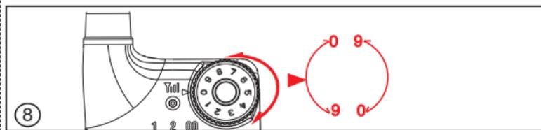
**Step 8:** Adjust the intensity of shock function by rotating the thumbwheel dial. 1-9 levels can be chosen. In level 0, you can do nothing with the remote.
