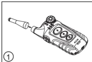
**Step 1:** Screw the antenna tightly onto the transmitter.
