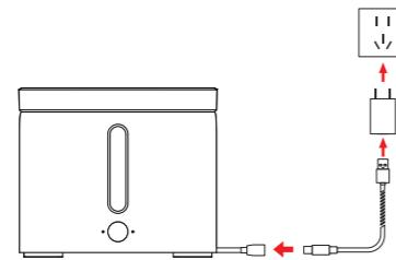
Please connect the USB power cord to the power port at the bottom of the main device and plug it into the power adapter interface. Finally, plug it in the power socket and turn on automatically.
