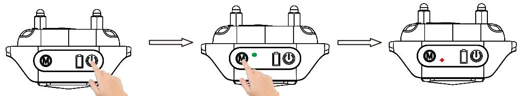
Power on the device by pressing and holding the Power Button for 2 seconds.
