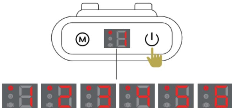
Press the power button (⏻) twice in succession to display number "1" on the screen (the product has been pre-set to automatic mode by default, where the function levels will be cycled from levels 1 to 6 automatically and no letter will be displayed on the screen.)
