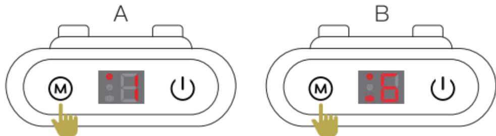
A.The product has been pre-set to the sensitivity level “**S**” by default before delivery. To adjust the sensitivity level, you may press the **M** button once. It is easier to activate the sensitivity level “**S**” than “**G**”.
