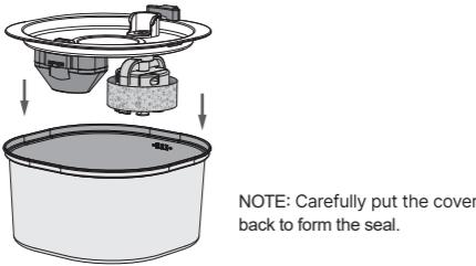
NOTE: Carefully put the cover back to form the seal.
