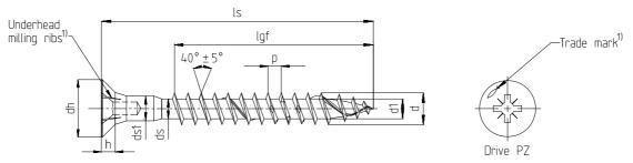
Power-Fast self-drilling screw - Countersunk headhole screw with full thread
