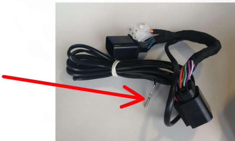
*This cable must reach the connector of the Magneti Marelli ECU which can be found next just above the transmission*
